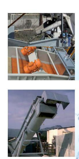
The mixers/trucks are washed and the residue is discharged into the screw separator or the dewatering screen.
