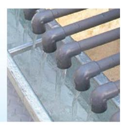
The filter press produces dry mud cakes (max 20% of residual moisture) completing more than 5 cycles per hour and reducing sludge volume by 80%.
