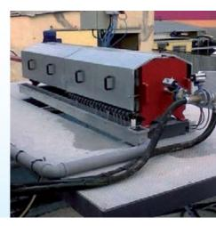
The filter press (D) filters the water by retaining all solids, returning completely clean water ready to be reused in the production cycle (E).
